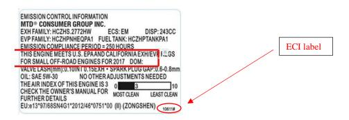
To conform to the statutory requirements, the label should state the following: "THIS ENGINE MEETS U.S. EPA EXH/EVP AND CALIFORNIA EXH REGS FOR SMALL OFF-ROAD ENGINES FOR (YEAR)."
